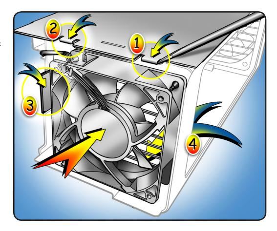
**4** Re-insert fan cables in clips on bottom of processor cage.
